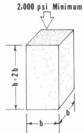
FIGURE 5 — Grout Prism.
