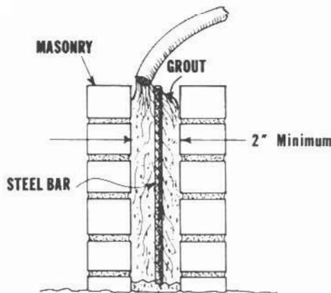
FIGURE 4 — Grout Being Pumped into Two-Wythe Brick Wall.
