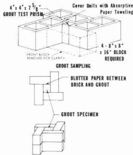
FIGURE 6 — Making Grout Prisms.
