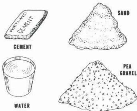
FIGURE 1 — Ingredients in Grout.
