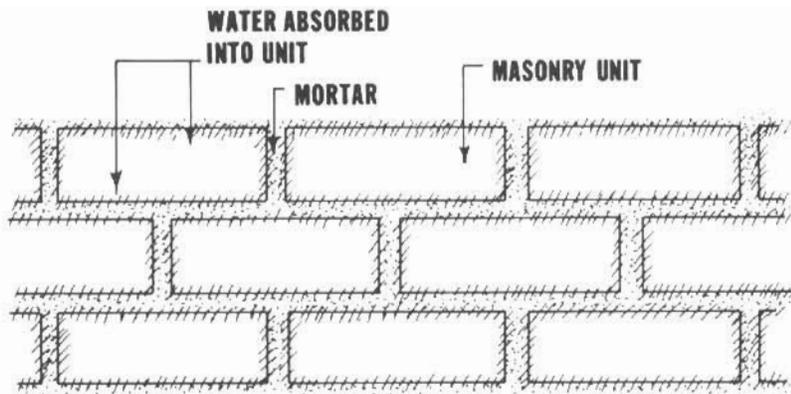
FIGURE 3 — Masonry Units Absorbing Excess Water from Mortar.
