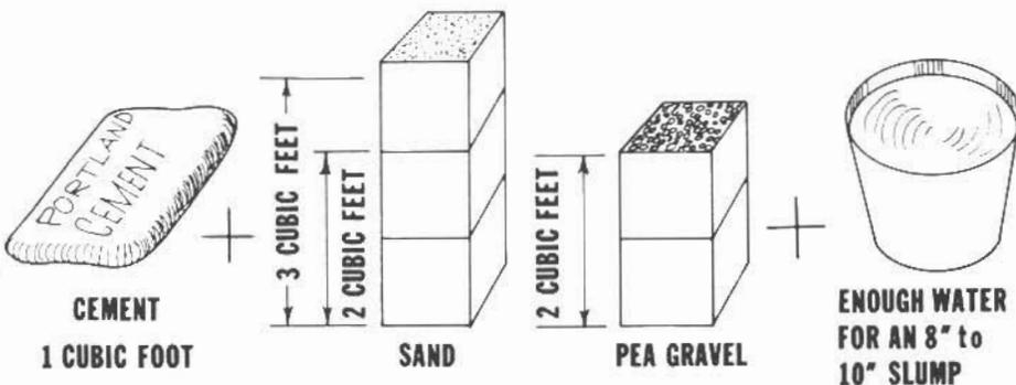
FIGURE 7 — Volumetric Proportions of Coarse Grout.
