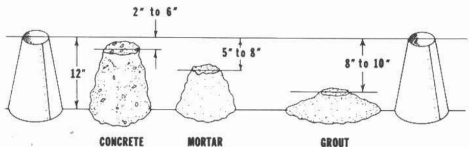
FIGURE 2 — Slump Tests of Concrete, Mortar and Grout.
