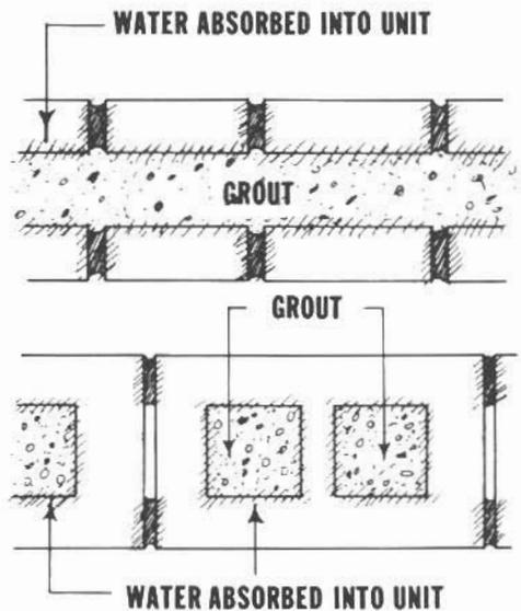
FIGURE 9 — Grout Spaces and Absorption of Excess Water by Masonry.
