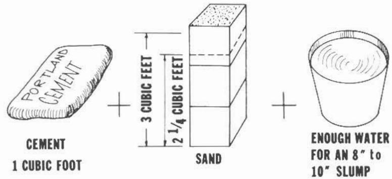
FIGURE 8 — Volumetric Proportions of Fine Grout.
